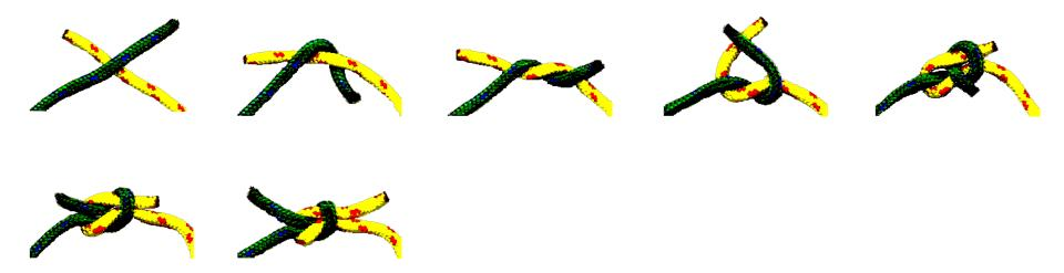
**Sheet Bend** – For joining together two pieces of rope of unequal thickness (securing a flag to the flag pole)
